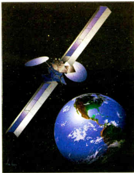
XM uses Hughes 702 satellites in a geostationary orbit.
