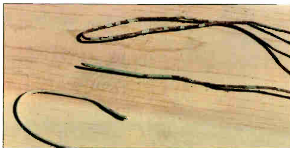
Fig. 1: Check the AM ground system for corrosion.
