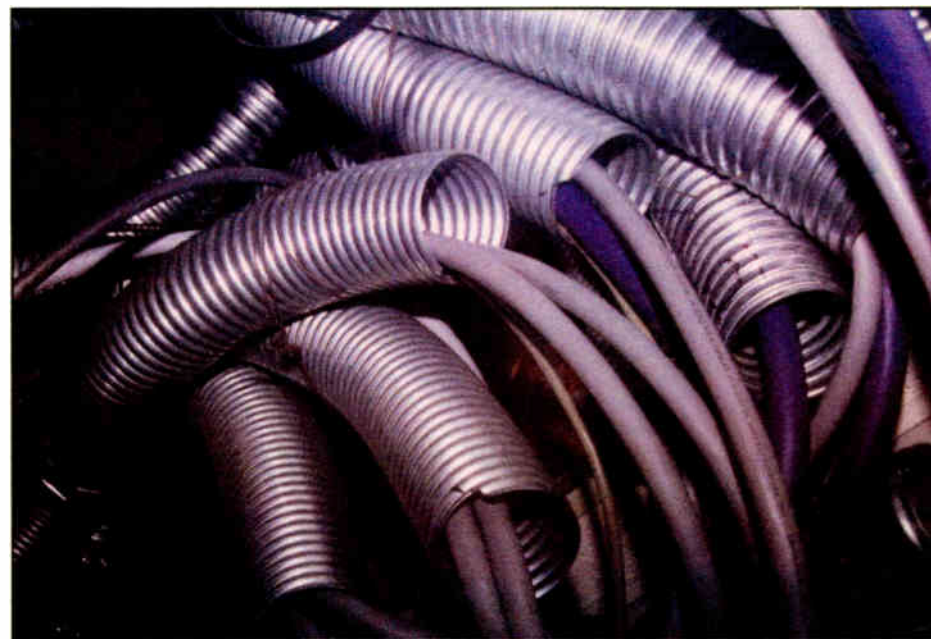
Fig. 4: Avoid this kind of armored conduit in your wire planning.
