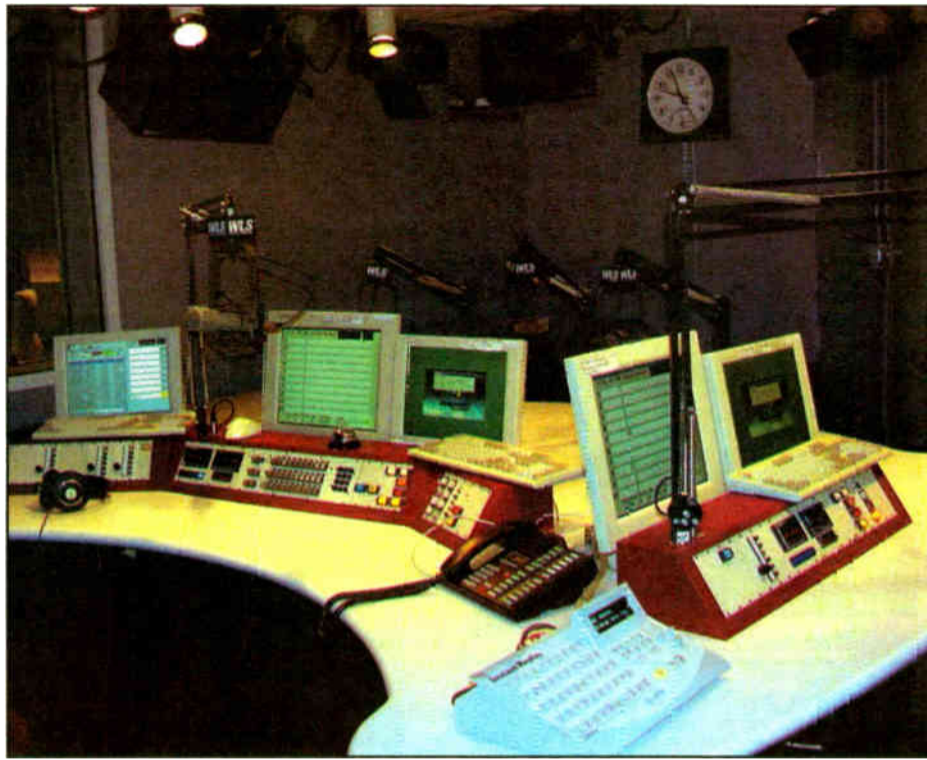
WLS(AM)'s Talk Show Setup on a Harris Hydraflex Desk
