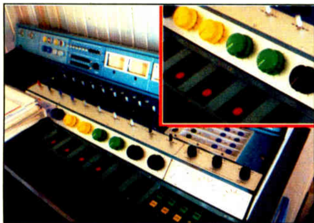
Consoles with large knobs that have distinctive positioning tabs for visually impaired users
