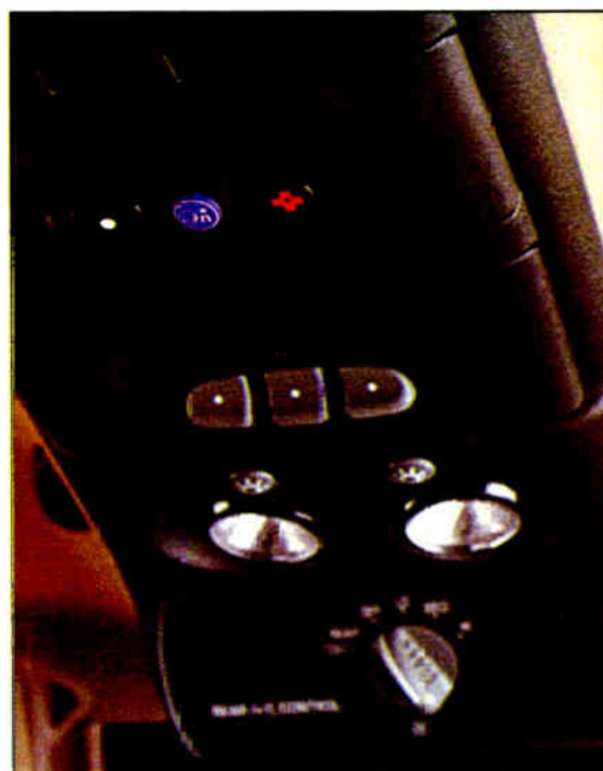
OnStar buttons can be integrated into the dash, rear-view mirror or ceiling (shown) — the car radio mutes when the OnStar buttons are used
