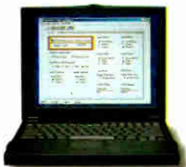
WHEATSTONE'S VDIP™ Virtual Dipswitch Software lets you configure our consoles with a laptop computer. There's no pulling cards, setting dipswitches or installing jumpers. Once configured the consoles run standalone.
