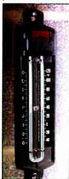
Figure 1: A high/low thermometer keeps tabs on transmitter building cooling.
