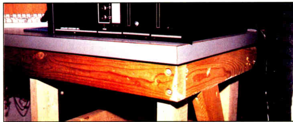
Figure 3: A 2x4 support frame was designed for the computer hard drive.
