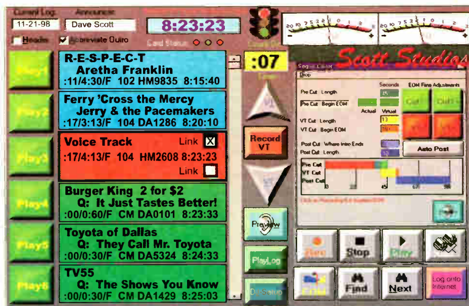
Here's Scott Studios' Voice Trax Via Internet (VTVI) software, shown with the optional Segue Editor. VTVI allows a distant announcer to pre-record a 4 hour show in about 15-20 minutes with nothing more than a Windows computer with an ordinary sound card, an Internet connection and a good microphone.
