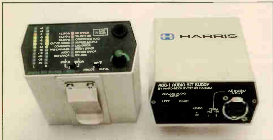
The Harris Audio Bit Buddy can trace and monitor a digital signal.
