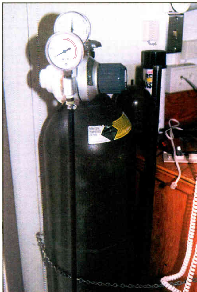
Figure 1: Inspect nitrogen tanks regularly and keep them chained to the wall for safety.
