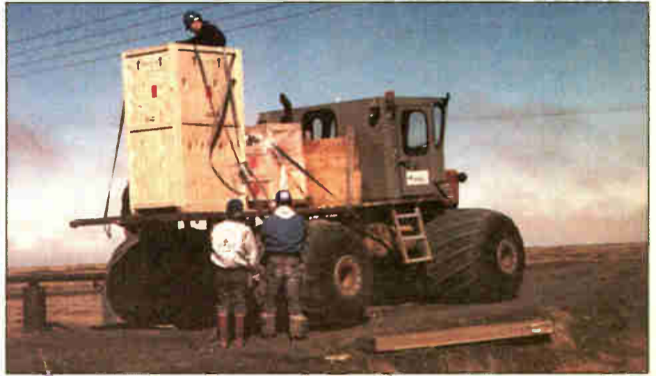
Travelling the last 1,000 feet of a long journey, a new Nautel transmitter moves through the tundra on a Rollagon.
