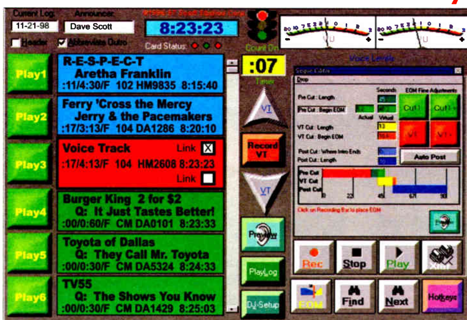
Here's Scott's Voice Trax Via Internet (VTVI) software, shown with the optional Segue Editor. VTVI allows a distant announcer to pre-record a 4 hour show in about 15-20 minutes with nothing more than a Windows computer, an Internet connection and a good microphone.
