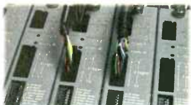
Fool-proof connectors prevent accidental circuit damage. Each input, output and logic connection is separate, so removal of one won't disable other signals and functions.
