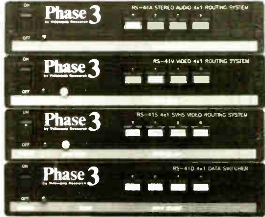
RS-41A 4x1 Stereo Audio Router, RS-41V 4x1 Video Router, RS-41S 4x1 SVHS Video Router, and RS-41D 4x1 Data Router
