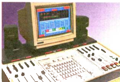
The 22,000 series console can add even more functionality to Trak*Star by providing video & audio monitoring, plus audio input & output feeds
