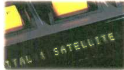
Each fader has a 10-character alphanumeric display. The display changes when another audio source is assigned, which can happen either manually or at a preassigned time.
