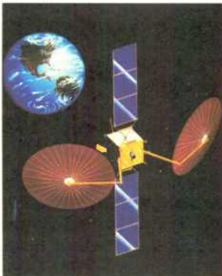
RadioSat would deliver two-way mobile digital radio using an MSAT satellite.
