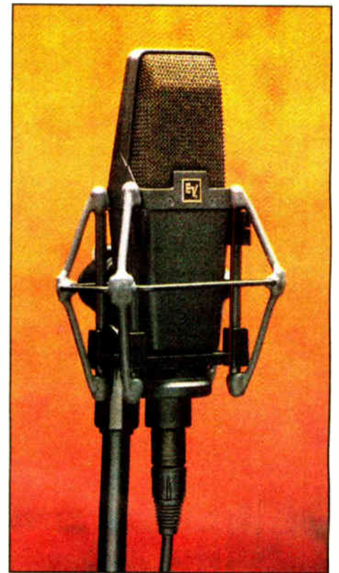
RE2000: ElectroVoice's cardioid condenser mic
