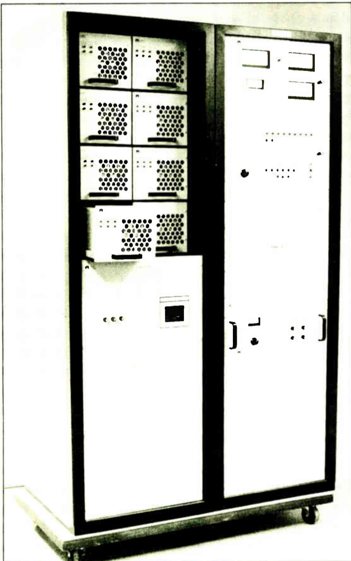
Totally solid state AMPFET ND 10 10kW AM
