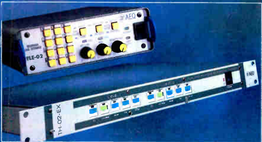
Digital Telephone Hybrid AEQ TH-02 EX
