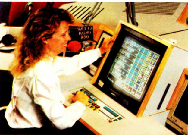
WCCO's uncluttered, paper-free Media Touch Minneapolis studio is shown above. Logs, timing, commercial outcues and live copy show on our screen.
