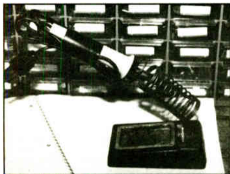
A plastic film container slipped over a soldering iron helps secure its cable.
