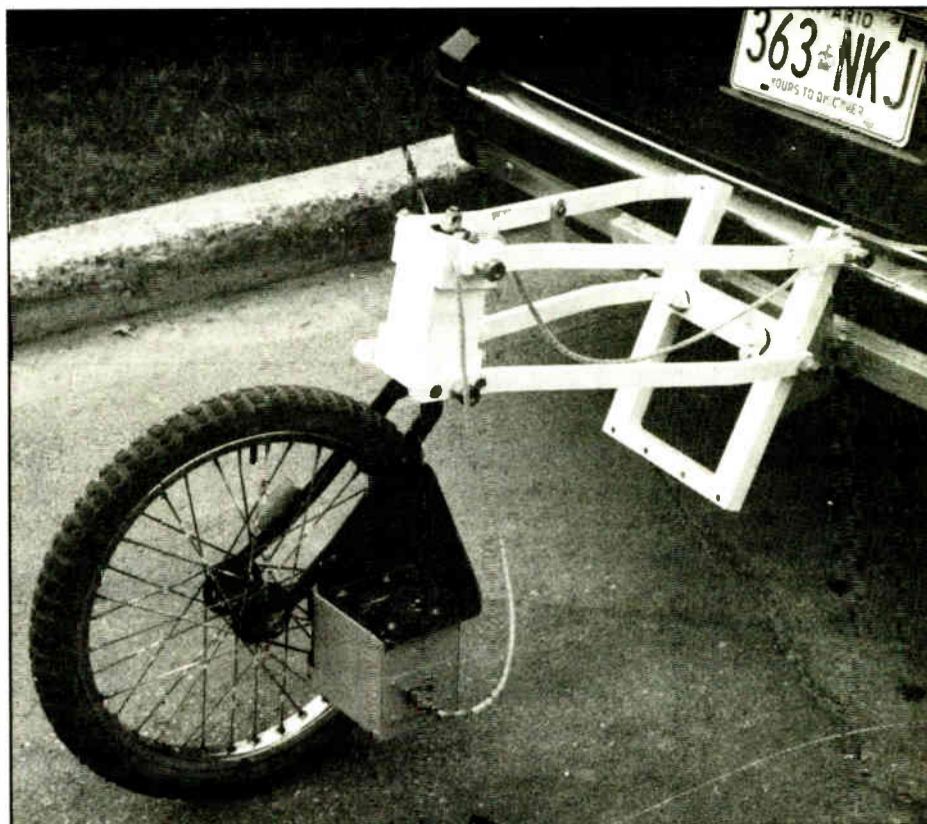
A special wheel-based system determines measurement intervals for the L-band tests.
