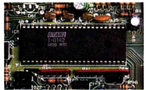
Because we know how hard you use our machines, we use a double-sided glass epoxy transport circuit board, and we silkscreen both sides of our PCBs so you can locate the components easily.
