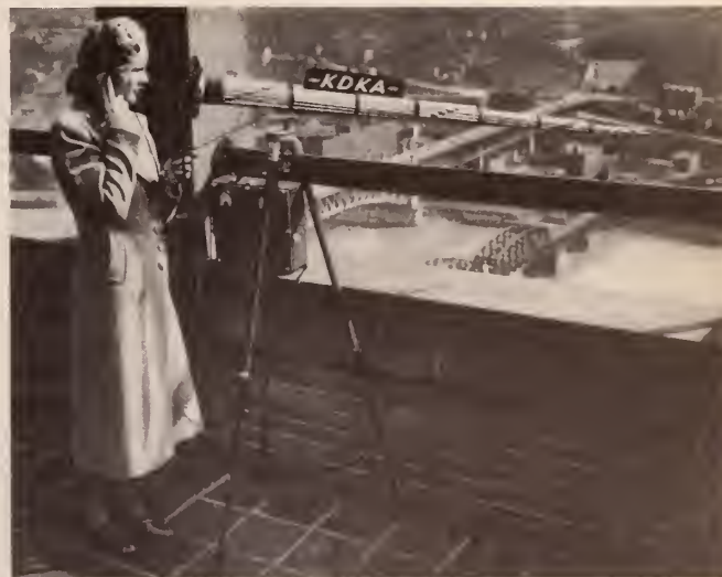
KDKA is using one of the new "Gatling Gun" microphones with much success on certain types of pick-up broadcasts. Station engineers took the "Gun" made of 52 small aluminum tubes to the roof of the Grant Building and trained it on a steamboat down on the Monongahela River. Viola Frazier, KDKA singer, put on the earphones just in time to hear the towboat whistle.
